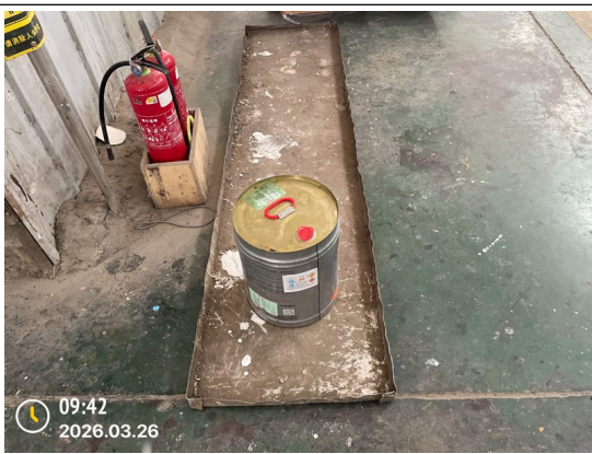
Chemical with secondary container and label
